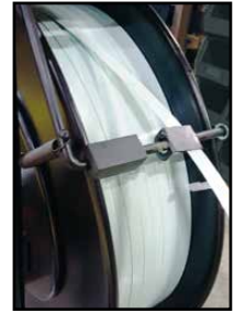
EXTRA HEAVY DUTY REEL BRAKE PREVENTS STRAP TANGLES RESULTING FROM THE COIL OVER SPINNING
