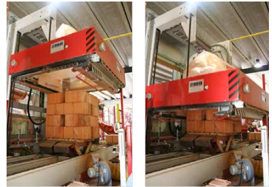
Hooder with Hot Air Thermoshrinking Device
