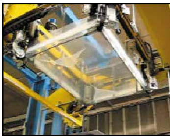
Film Stretching (Note: "Dog ears" or "elbows" are inside the hood)
